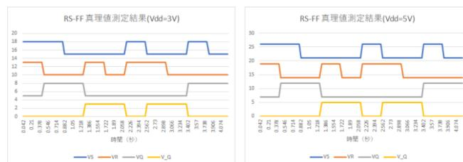
Fig. 3 R-S Flip-Flop input-output waveforms
