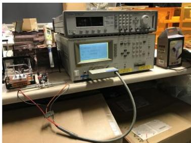
Fig. 1 Measurement the permittivity by LCR meter
