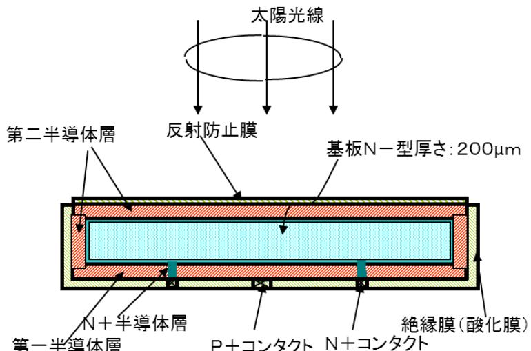
Fig. 1 Cross-sectional drawing of a new type solar cell
