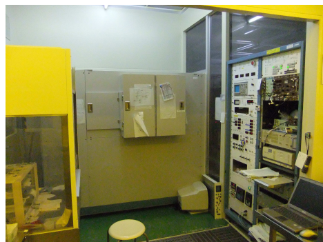
Fig. 1. Ion implantation machine. Use of high temperature implantation will be examined from year 2014.
