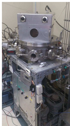
Fig. 1. Photograph of PECVD (Plasma Enhanced Chemical Vapor Deposition)
